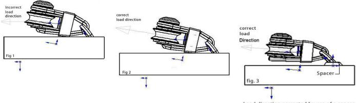
Load direction corrected by use of a spacer.
