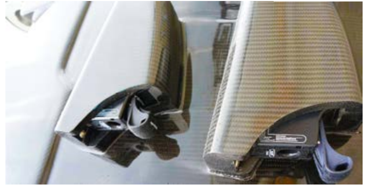
Above: an example of the detailing incorporated on the Future Fibres' mast. As well as these jammer housings, custom built steps are fitted near the base
